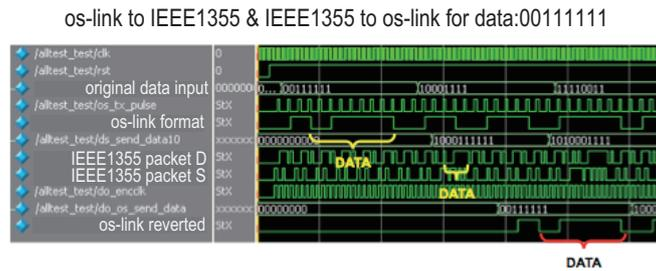
Figure 4: Time sequence of OD convertor. From a TPCORE, data:00111111<sub>2</sub> in os-link format is inputted, and converted to IEEE1355 protocol in an OD convertor, and this chart shows also data reverted to os-link format.
