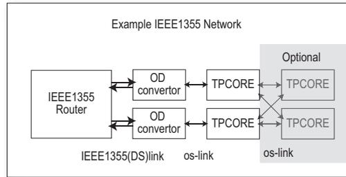
Figure 2: The example network setup with two (four) TPCOREs
