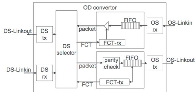
Figure 3: Block diagram of a bi-directional OD convertor (IEEE1355  $\rightleftharpoons$  os-link)
