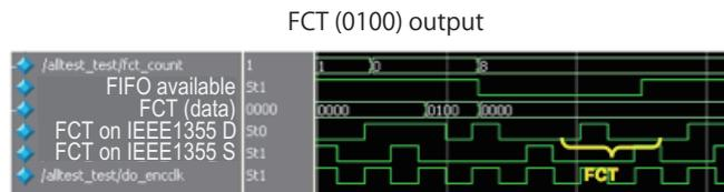
Figure 5: Timing chart to demonstrate the functionality of FCT transmission. If output FIFO for DS to os-link conversion part of an OD convertor has a room to accept data (FIFO available high), then FCT signal (bit sequence 0100<sub>2</sub>) is transmitted over DS-link to prompt the data transmission side to send further eight tokens.
