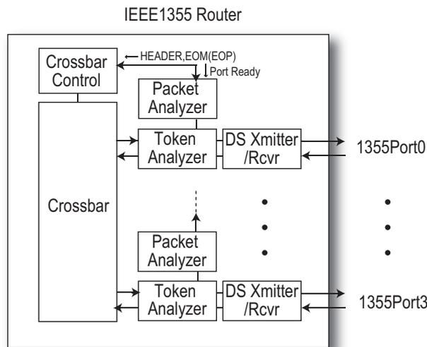
Figure 1: Block diagram of presently developed IEEE1355 Router
