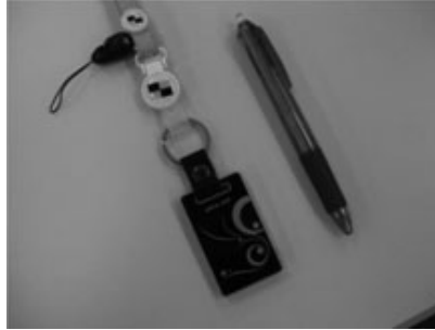
Fig. 2. A GPS logger used for our survey (Qstarz Black Gold 1300)
