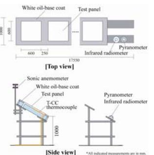
Figure2. Diagram of the test panel platform
