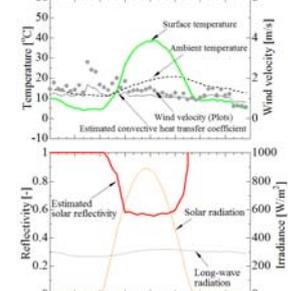
Figure10. Fluctuation of the estimated solar reflectivity on a typical, clear day
