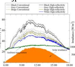
Figure9. Fluctuation of surface temperature of each test panel on day 20 with typical, clear weather.
