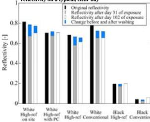
Figure11. Spectral reflectivity (diffuse and specular component) of the high-ref paint
