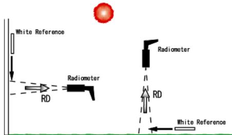
Figure 4 Diagram of measuring spectral reflectivity in the actual condition
