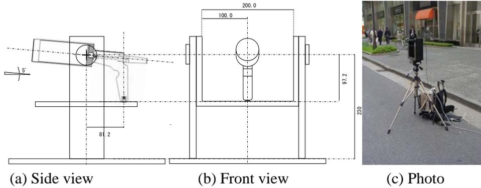
Figure 6 Diagram of the mechanical platform for 1 degree FOV
