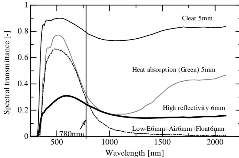
Figure 2 Spectral transmittance of the glasses available commercially
