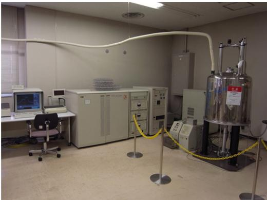
Figure 2. A nuclear magnetic resonance spectrometer for analyzing the chemical forms of carbon, nitrogen and phosphorus contained in seabird excreta
