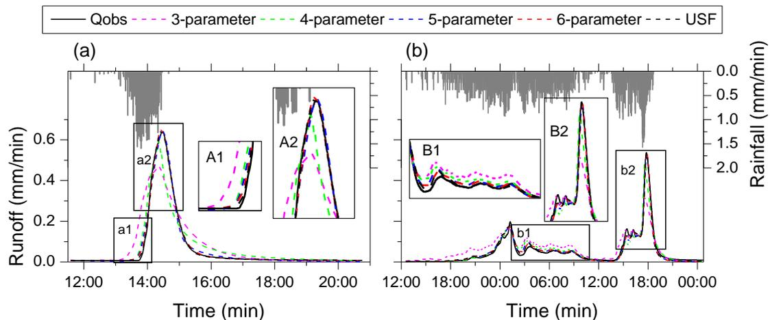
**Fig.2** Reproduced hydrograph by each model for (a) Event 1 and (b) Event 3. The rectangles A1, A2, B1, and B2 represent the enlarged view of the sections a1, a2, b1, and b2 of the hydrograph.
