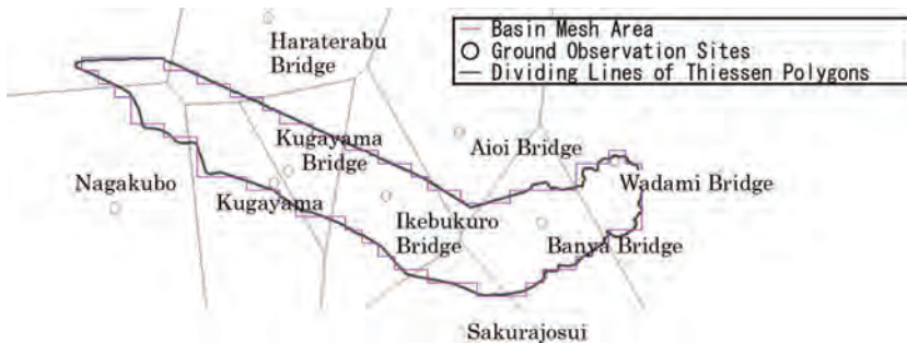
Figure 7: Mesh area of the target basin.
