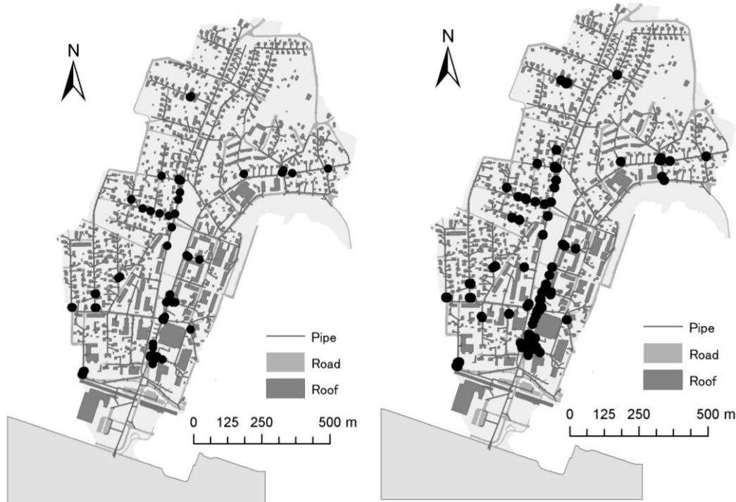
Figure 6. Flooded manholes for today's design storm (a) and future design storm (b).
