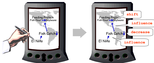
Fig. 1. A pen-based system, where users employ arrow symbols while sketching or annotating their ideas or plans on the screen as naturally as people often do on papers in face-to-face communication. When processing such diagrams, the system must interpret the semantic roles of the arrow symbols.
