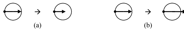
Fig. 6. Smooth transitions between two DLine-region relations, derived by moving the DLine's ending point from the region's boundary to (a) interior and (b) exterior, respectively. In (b), the movement of the DLine's ending point generates the intersection of the DLine's interior and the region's boundary.
