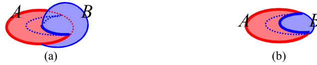
Fig. 1. Configurations of two contact relations, derived from the topological region-region relations in (a) Fig. 8U 1 and (b) Fig. 8e 1 , in which the region A is clipped by the region B
