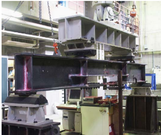
Photograph 3. Test setup of loading system.
