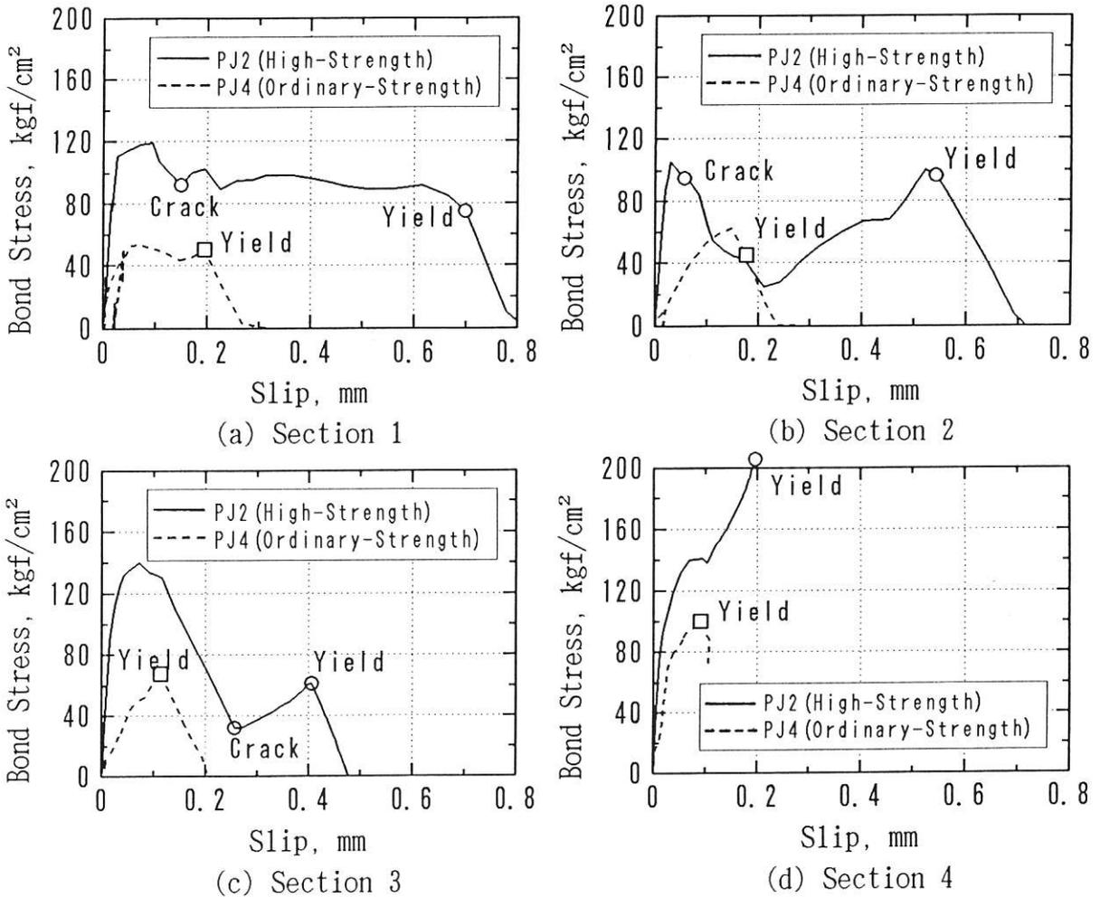
Fig. 7 : Bond Stress – Slip Relations in Each Section
