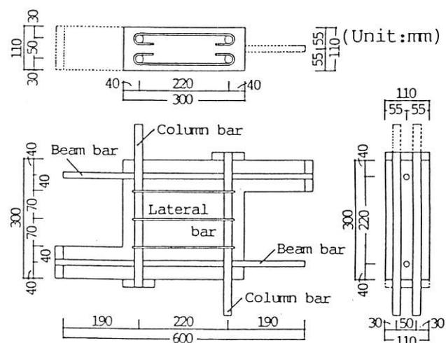
Fig. 1 : Reinforcement Details
