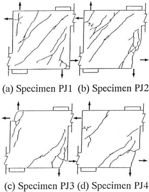
Fig. 3 : Crack Patterns after Test
