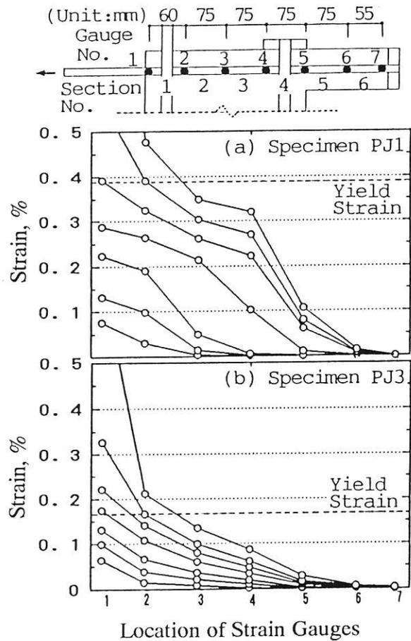
Fig. 4 : Strain Distributions along Beam Bar
