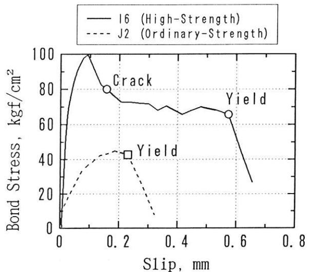
Fig. 8 : Bond Stress – Slip Relations in Beam–Column Joint Specimens
